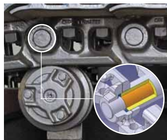
Tracks The chain is composed of self-lubricating sealed links isolated from all external contamination. The tracks are locked by mechanically bolted pins.
